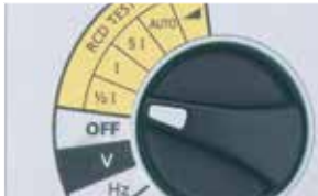
Clear range selector for poor light conditions
