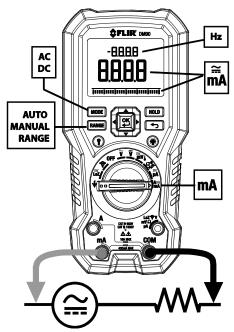
Fig. 5-9 mA Current and Frequency Measurements
