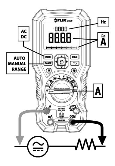
Fig. 5-8 High Current 'A' and Frequency Measurements
