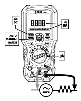
Fig. 5-10 uA Current Measurements
