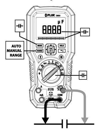
Fig. 5-5 Capacitance Measurements
