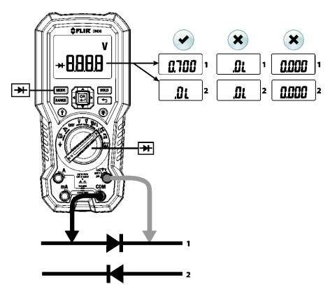
Fig. 5-3 Classic Diode Measurements
