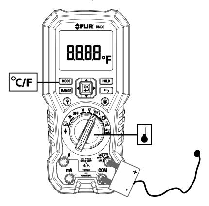
Fig. 5-6 Temperature Measurements
