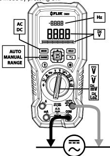
Fig. 5-1 Voltage and Frequency Measurements
