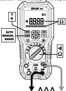
Fig. 5-2 Resistance and Continuity Measurements
