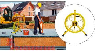
Using a fibreglass locating cable allows you to reliably find the exact position of sewers and PE ductworks. Depending on the connection to the Easyloc TX transmitter, either the entire route can be located or just the tip of the cable. The fibreglass locating cable is available in a large variety of lengths.
