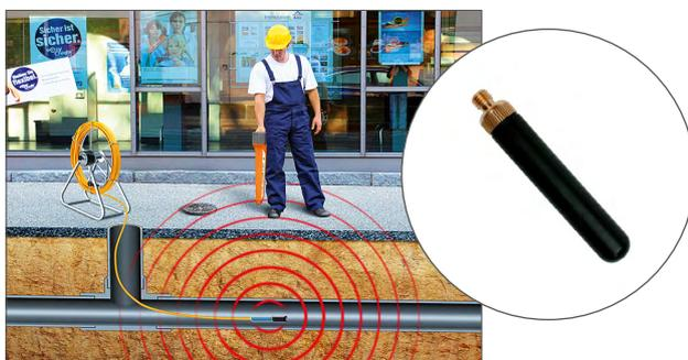
The MLS 55-3 pipeline transmitter probe is a slim, battery powered mini-transmitter and has a range of 5 m. When attached to a drain rod or fiberglass push rod cable by one of the 3 adapters provided, it is used to locate ductworks or blockages. A heavy duty protective cover is available.
