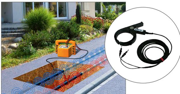
The Easyclamp transmitter clamp is used to send the 33 kHz signal onto and along live cables without shutting off their power. The Easyclamp is connected to the Easyloc TX transmitter and installed around the cable, providing effective route tracing.
