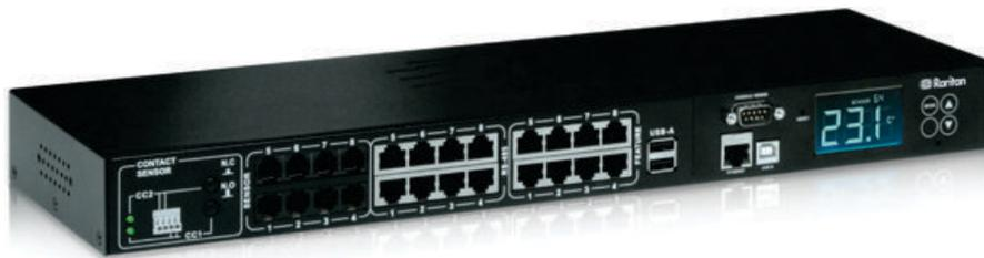
Raritan's environmental rack controller is an IP-based appliance that allows you to use any of Raritan's sensors such as temperature, humidity, air pressure and airflow
